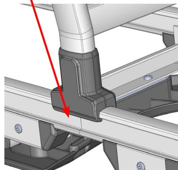
d: Centre leg positioned to fit between tub and toilet
