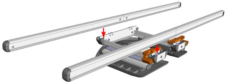
b: With seat opening facing towards you, turn seat upside down. Lower rails onto rollers
