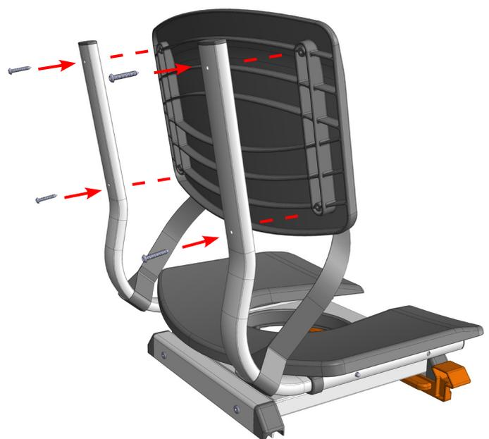
Fit seatback to seatback tubes with screws provided
