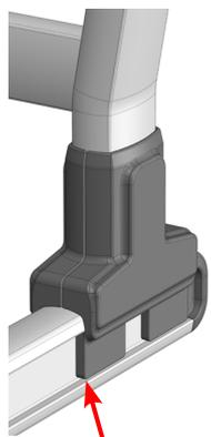
f: Check if the clamp is fully engaged (no gaps between the clamp & the rail)
