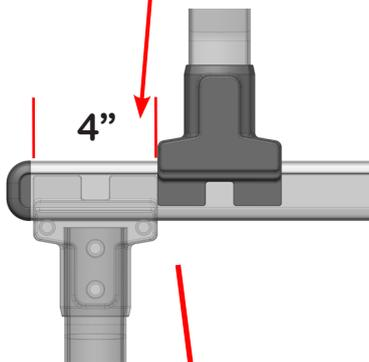
e: Locate leg 4" (100mm) from rail end to allow for grab bar
