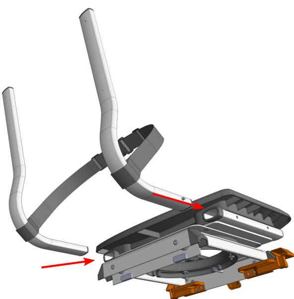
Fit seat belt to seatback tubes and slide into the seat tubes
